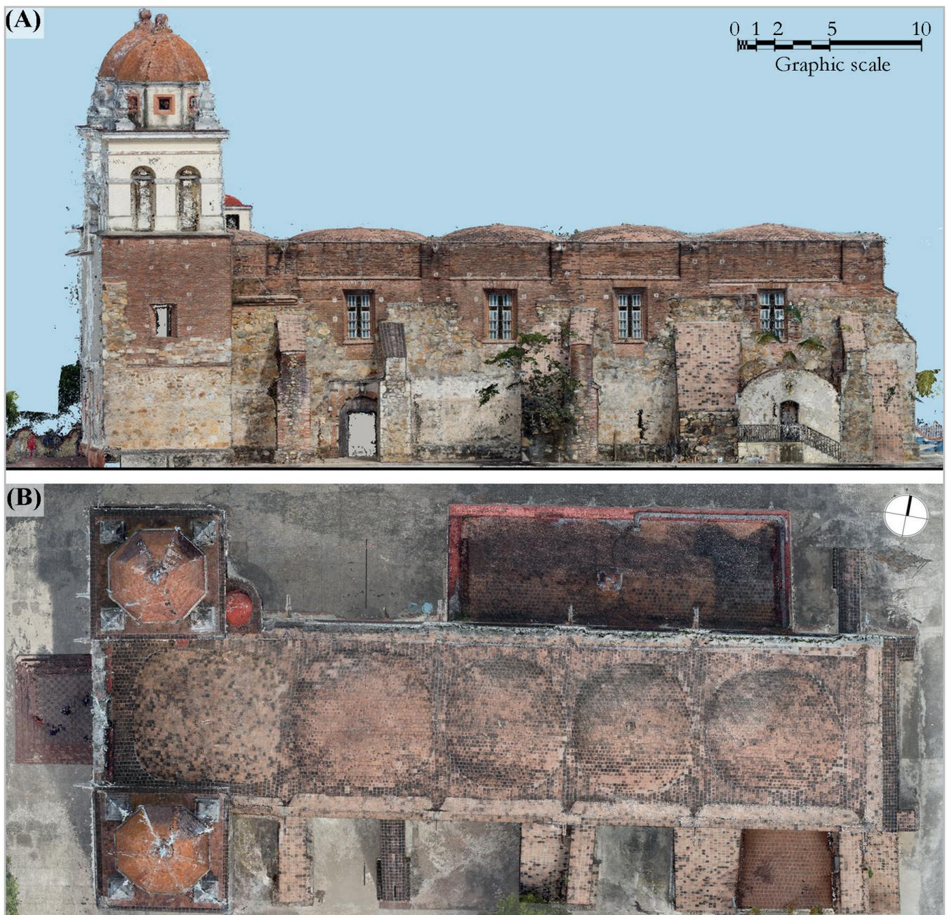
**Figure 6.**- Clean point cloud, within the SketchUp software, perpendicular views: (A) south elevation view and (B) rooftop plan.
